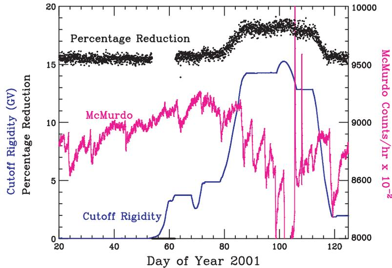
**Figure 4.** Time profile plot of the 2000–2001 latitude survey north bound voyage. The points show the percentage of counts having  $\delta T < 1200 \mu\text{s}$ . The McMurdo count rate provides an indicator of solar activity during the survey. The effective vertical cutoff rigidity is shown as a solid line. Flat regions of the solid line occur when the ship is moored. The data are hourly averages.
