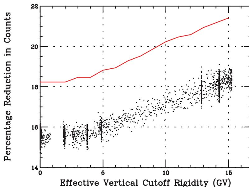
**Figure 5.** Observed percentage of counts having  $\delta T < 1200 \mu\text{s}$  as a function of effective vertical cutoff rigidity. The curve is the result of our simulation.
