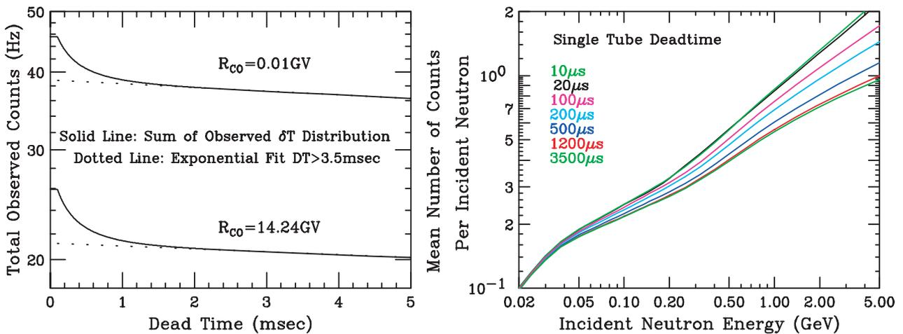
**Figure 3.** (left) The integral of  $\delta T$  distributions shown in Figure 1 as a function of the integral lower limit. The integral is the neutron monitor count rate when the dead time is the integral lower limit. (right) The average number of counts in a 6 tube NM-64 calculated for different dead times.
