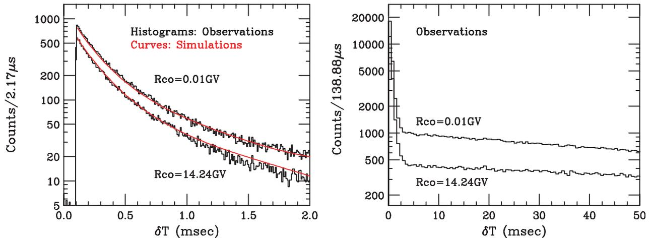
**Figure 1.** (left) Distribution of the elapsed time  $\delta T$  (modulo 142 ms) between measured single tube counts for 14.2 GV cutoff rigidity (lower curve and data) and 0.01 GV cutoff rigidity (upper curve and data). The histograms represent the observed data. The curves represent simulated data scaled by a factor of 0.7. (right) The same data on a compressed scale illustrating the transition from correlated to uncorrelated counts.
