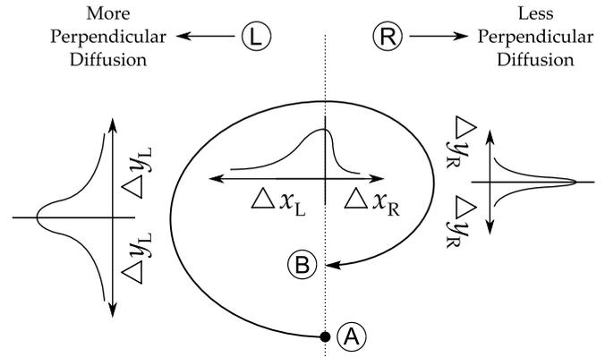
FIG. 12.—Particle orbit from point A to point B depicts the origin of classical (antisymmetric) gradient drift. The Gaussian distributions at left and right display the source of residual antisymmetric drift. Finally, the asymmetric distribution in the center depicts the origin of symmetric drift arising from the nonuniform perpendicular diffusion coefficient. See text for further details.
