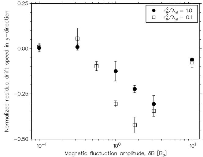
FIG. 10.—Residual antisymmetric drift speed in the  $y$ -direction for  $r_M^0/\lambda_{\text{sl}} = 1.0$  and  $r_M^0/\lambda_{\text{sl}} = 0.1$ . The residual is normalized to the weak-scattering value of the drift speed in the  $y$ -direction.
